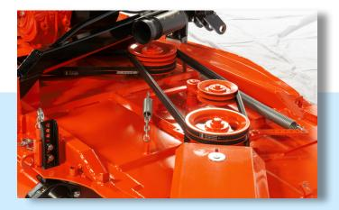
The heavy v-belt transmission with autometic tensioning ensures an excellent capacity, also in tall grass.
