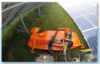
Because of its large offset in combination with the swing arm, the RF mower is very well equipped to mow the grass between and underneath solar panels and to cut grass under board fences, along wire or rock fences and around fence posts.
